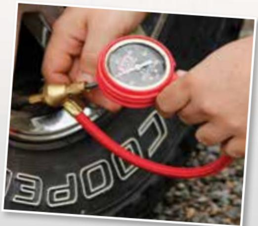
to build up which could lead to tyre failure. Low pressures increase rolling resistance, causing a reduction in fuel economy. You would also find a significant loss of steering precision and cornering stability. While an under inflation of 6psi, as an example, doesn't seem like much, it usually **represents about 20%** of the tyre's recommended pressure. You should also be aware that the load capacity of your tyres is reduced at lower pressures.
